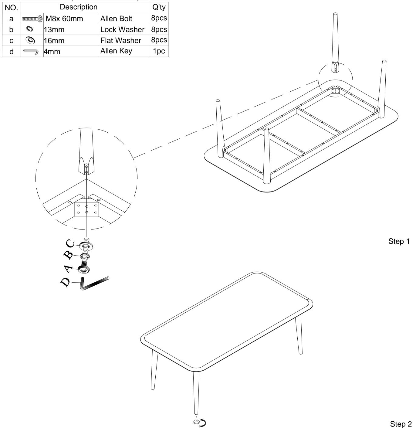
Note: Do not fully tighten the bolts untill all parts are in place. Failure to follow these instructions may cause the bolts to misalign during assembly.
